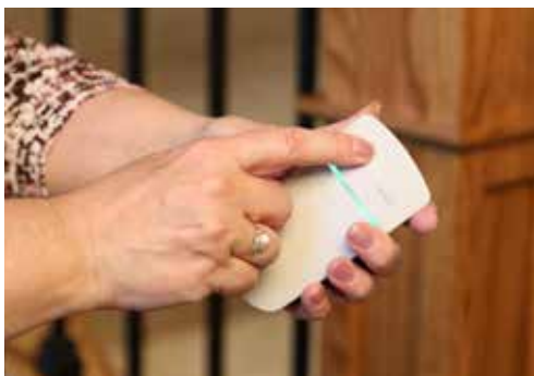
Two wireless call/sends allow remote control access.
